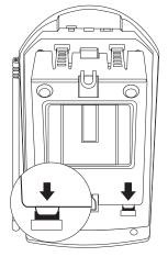
Plug the AC Power Cord (1) and the Telephone Line Cord (2) into the base.
